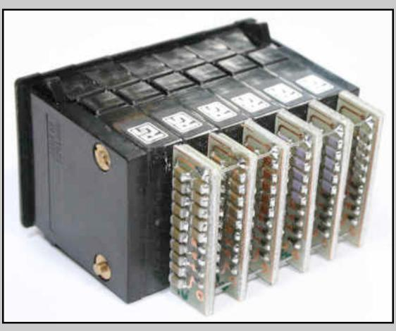
The decades are bussed together with wires passing through the switch common pin, and the common on the PCBs. I drilled an extra hole in the thumbwheel PCBs to allow the second wire to pass through neatly.
