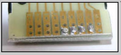
The four switch contacts are pinned through and soldered
