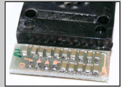
A small PCB with fifteen 1206-size ceramic caps fitted neatly on the back of the switches I used.
